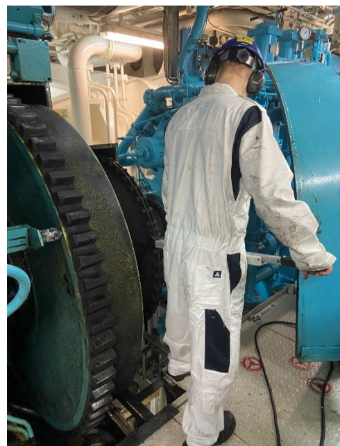
Retrofitting Main Engine Centa Flex coupling with Metapower sensors, the cabinet with the HSI0 processing module and 7" display in Engine Control Room.
