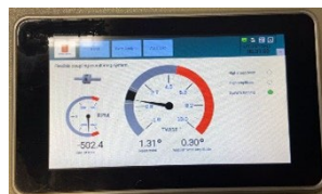
Retrofitting Main Engine Centa Flex coupling with Metapower sensors, the cabinet with the HSI0 processing module and 7" display in Engine Control Room.
